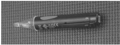
Figure 28 - Non-Contact Circuit Tester
