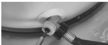
Figure 26 - Drain Valve
